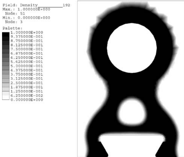
Fig. 13 Multiple-load case, minimum energy problem. Final density
